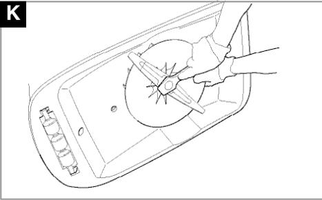
**Always handle the blade with care - sharp edges could cause injury. USE GLOVES. Never use more than 3 Cutting Height Spacers. Spacers must only be fitted between the blade and the fan and NEVER between the blade and the bolt.**
